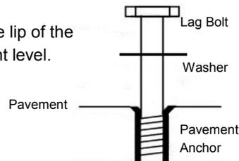
Using a 9/16" socket, tighten the bolt until washer is firmly seated. **DO NOT over tighten**
